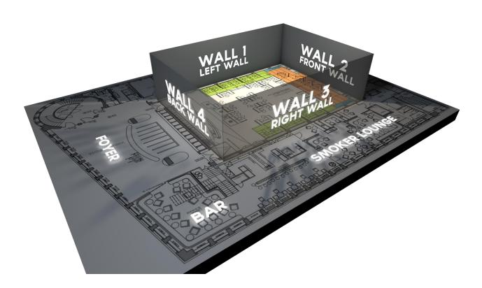
For the overview and production the entire screen is divided on four walls. The term "WALL 1 to 4" is used from production to implementation.
